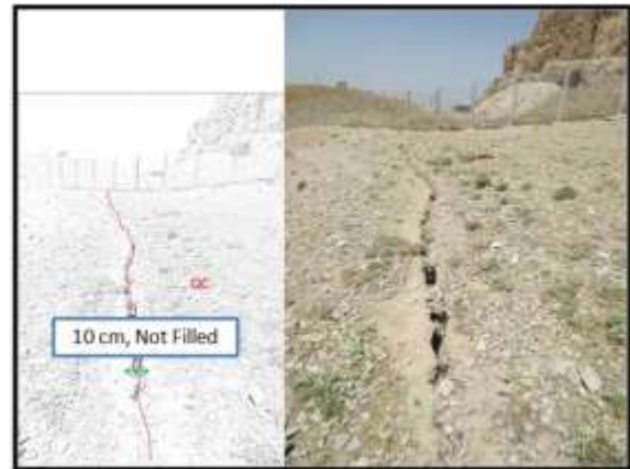
Figure 13: new movement because of Naghshe Rostam fault in quaternary alluvium (view 240°)
