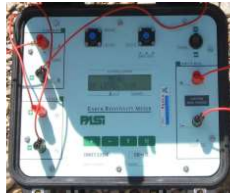
Figure 4: it indicates the geophysical device PASI whose model is GL -16. Contribute a better translation
